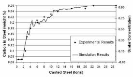
Fig. 5: Carbon content during a steel change situation in tundish with flow control device.
