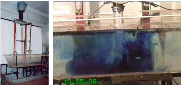
Fig. 1. Experimental tundish model used in the present investigation
