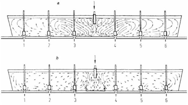
Fig. 4. Flow patterns in the six-strand tundish: a) no dams applied; b) lower dams applied in the incoming area.
