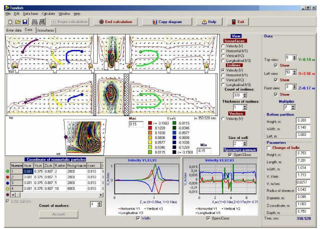
Fig. 3. TUNDISH program window: estimated values for steel flow in the sixstrand tundish
