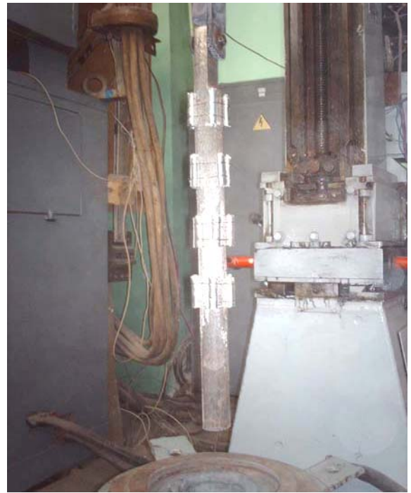
Figure 3: Scheme of disposition of metallic calcium portions on electrode during fulfillment of experiment on A-550 furnace.
