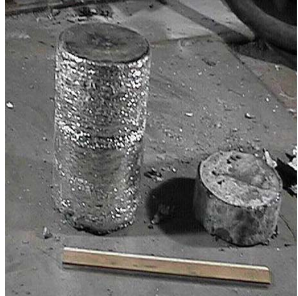
Figure 4: View of lateral surface of ingot after ESR with oscillations.
