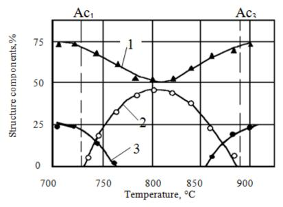
*Fig. 1. Amount of structure components in 10HSND steel after cooling on air from different temperatures of intercritigal range: 1 - ferrite, 2 - bainite, 3 – pearlite*
