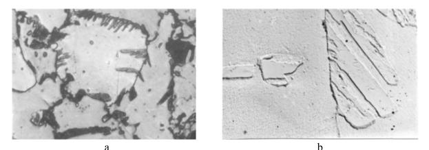
Fig. 2 Oriented formation of austenite in normalized steel 10HSND at 780°C a - x1000, b - x4200
