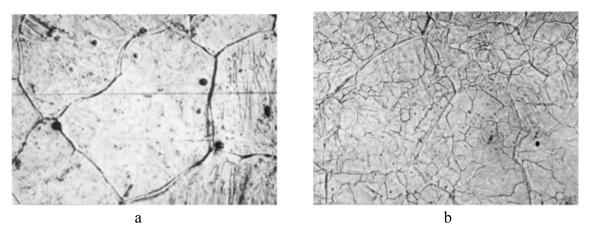
*Fig. 3. Change of austenite grain previously overheated (1050 °C) 10HSND steel at repeated heating to 930 °C after preliminary cooling to 750 (a) u 600 °C (b), x 400*
