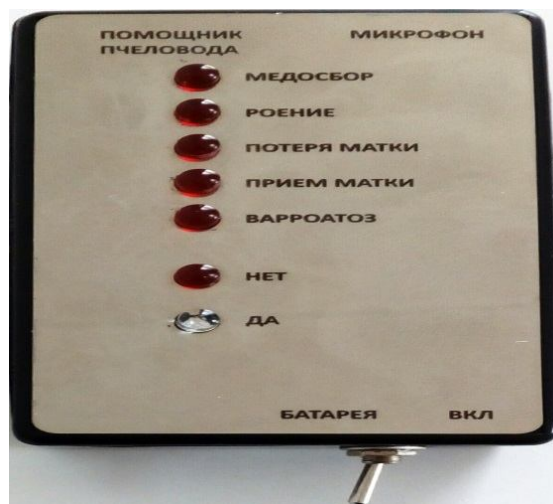
Fig. 2. The device for acoustic control of a condition of bee family in the form of implementation
