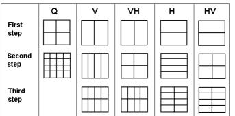
Figure 2. Different variants of space devision for image encoding on the basis of 2D tetracode.
