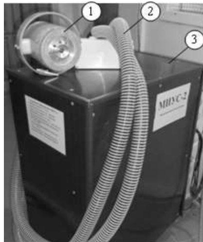
Figure 2 — The experimental complex for the electromagnetic flattening of the automobile steel body, the complex in the whole: 1 – is a tool for flattening; 2 – is the cable connection; 3 – is the power source (MPIS – 2, “the magnetic pulsed installation on 2 kJ”
