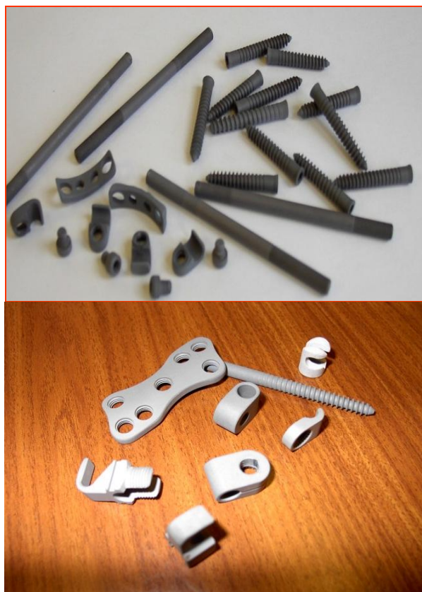
Fig. 9. Samples of implants for interbody spinal fusion with installation tool coated by oxide-ceramics formed in activated electrolytes
