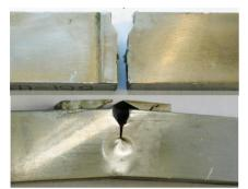
**Fig. 1.** Brittle fracture of the sample from group I (upper) and plastic deformation of the sample from group III (lower).
