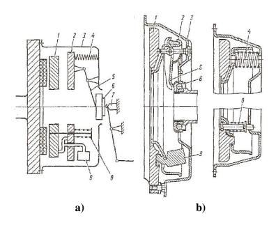
Fig. 14. Centrifugal Clutch: a) scheme b) arrangement
