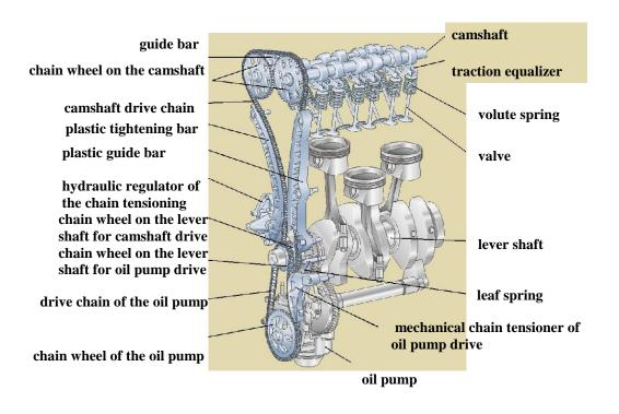
Fig. 13. Skoda's cam drive and oil pump drive of the 4-valve engine
