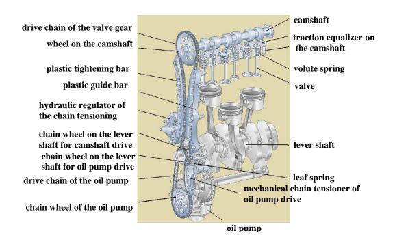
Fig. 12. Skoda's cam drive and oil pump drive of the 2-valve engine
