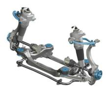
Fig. 16. Front suspension
