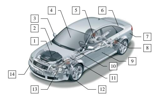
Fig.15. Basic components and units of the automobile
