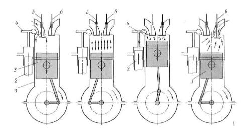
Fig. 11. A four-stroke cycle
