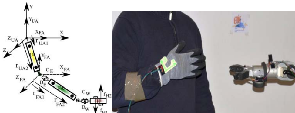
Figure 1 – Anthropomorphic arm coordinate systems and image of a human hand equipped by triaxial acceleration sensor and KATANA 450 robot of the ETIS laboratory, France with FSR sensors installed.
