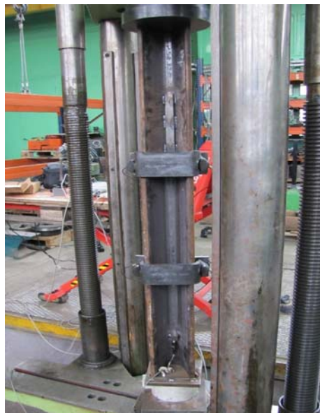
Fig. 3. Method of assembly the frictional joint with the resistance wedge at the static compression
