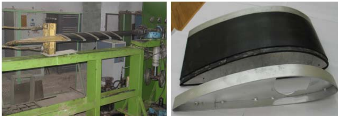
Fig. 2 Blade with flexible elements and rib
