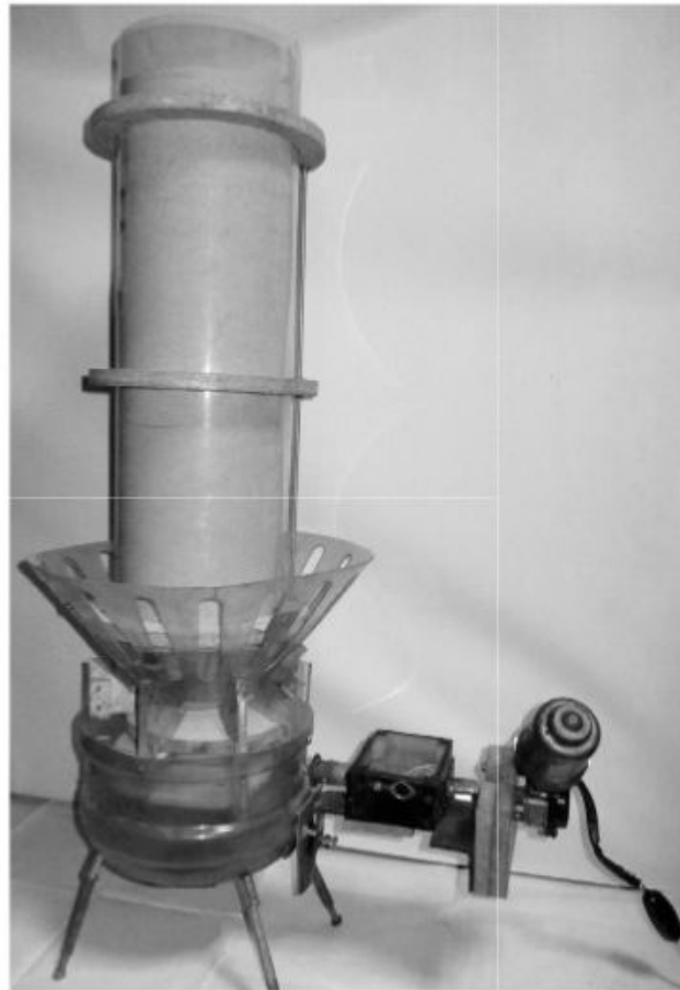
Fig. 4. Physical model of the system of unloading of lime from the shaft burning furnace with strain-gauge transducer mounted in the kinematic chain of the drive for the monitoring of changes in the torque.
