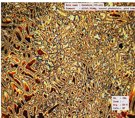
Fig. 3 AlZn5,5Cu2,5Mg1,5 alloy microstructure before homogenizing annealing, metallic form, enl.: ×100
