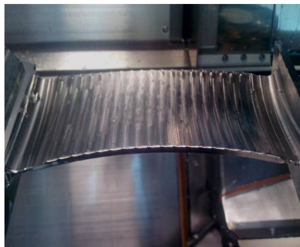
Fig. 7. Exterior view of the workpiece after semi-finishing blade milling
