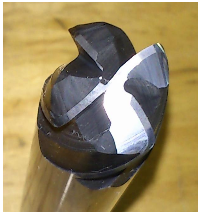
Fig. 4, b) HALTEC end mill series HFM after 120 minutes machining
