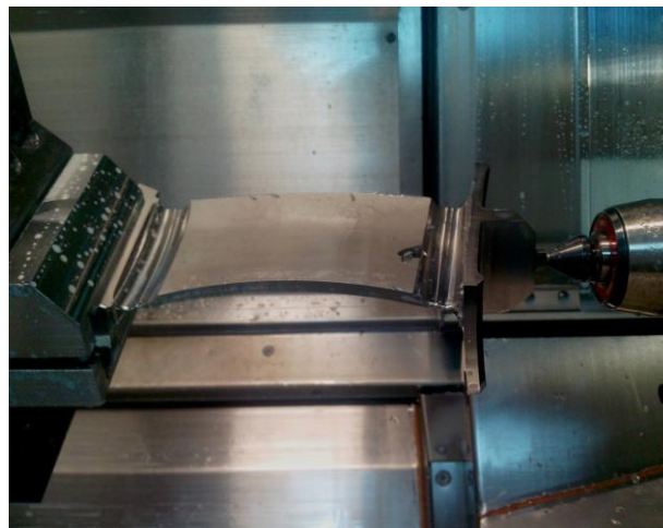
Fig. 6. Blade workpiece in the machine device
