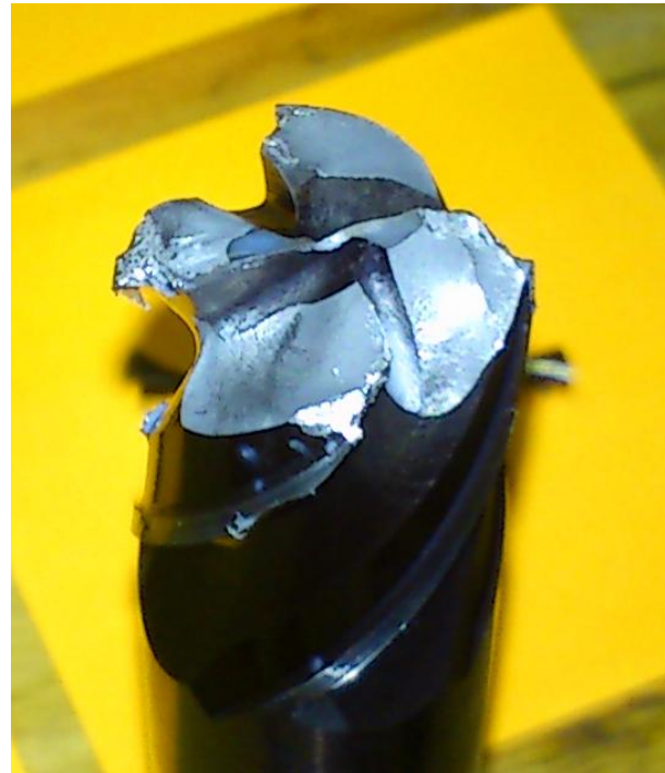
Fig. 4, a) SGS end mill series ZAPCR after 6 minutes machining
