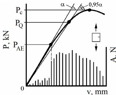
**Fig. 2.** Intensity change of the acoustic emission signals at point  $P_{AE}$  as a criterion for the macrocrack propagation.
