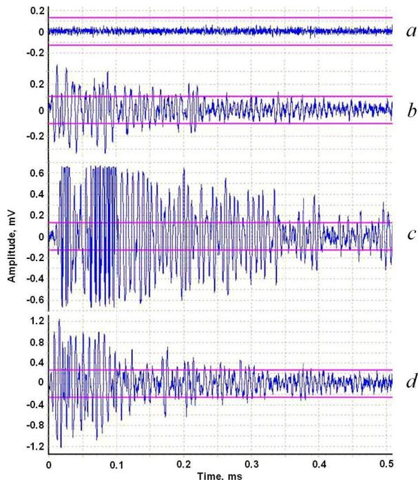
**Fig. 3.** Acoustograms recorded by the AE system SCOP-8 during experimental studies: *a* – background noise of the system; *b* – typical early signal for the samples representative of the group I and II; *c* – typical acoustic signal in the vicinity of  $P_{AE}$  (fig. 2); *d* – representative acoustic signals when the load approaches  $P_Q$  (fig. 2).
