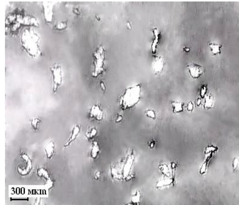
Fig. 1. Overview of alloy AK12MMgN powder wastes microparticles after regeneration (on plastic plate), ?32.
