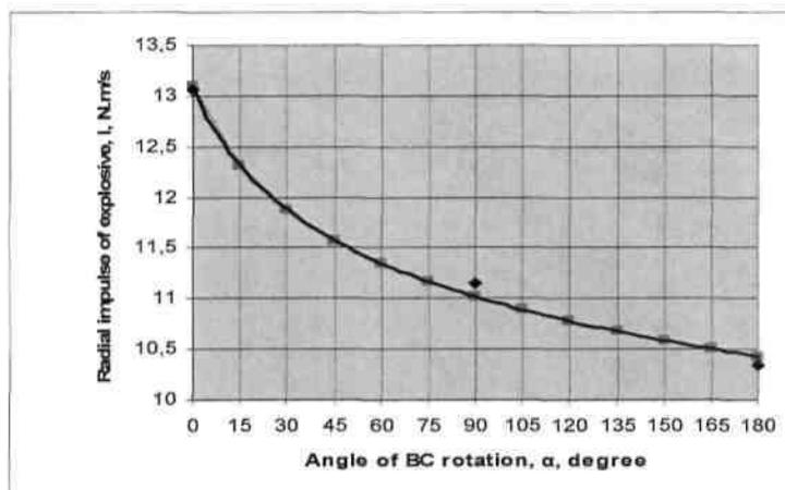
Fig.3. Functional depending of radial impulse of explosive from the angle of CR rotation
