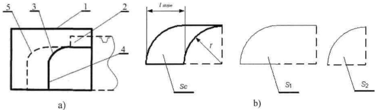
Fig.1. A curve terraced form of the excavation's working face: a) general form; b) schemes for a calculations of the squares of a curve part of an excavation
