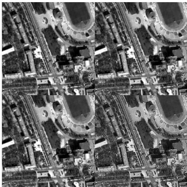
Figure 5 - Result of image fusion (from left to right and from top to bottom - WA, IHS, HDWT, DDWT)
