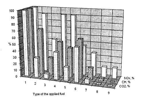
Figure 1 – Comparative estimation of the influence of alternative types of fuel on the ecological characteristics of motor-car engines with the forced self-ignition: 1- petrol; 2 - petrol + products of its conversion; 3 - petrol + H<sub>2</sub>; 4 - pressed oil gas; 5 - compressed natural gas; 6 - methanol; 7 - methanol +H<sub>2</sub>; 8 - synthetic gas (H<sub>2</sub> + CO); 9 - hydrogen (H<sub>2</sub>)
