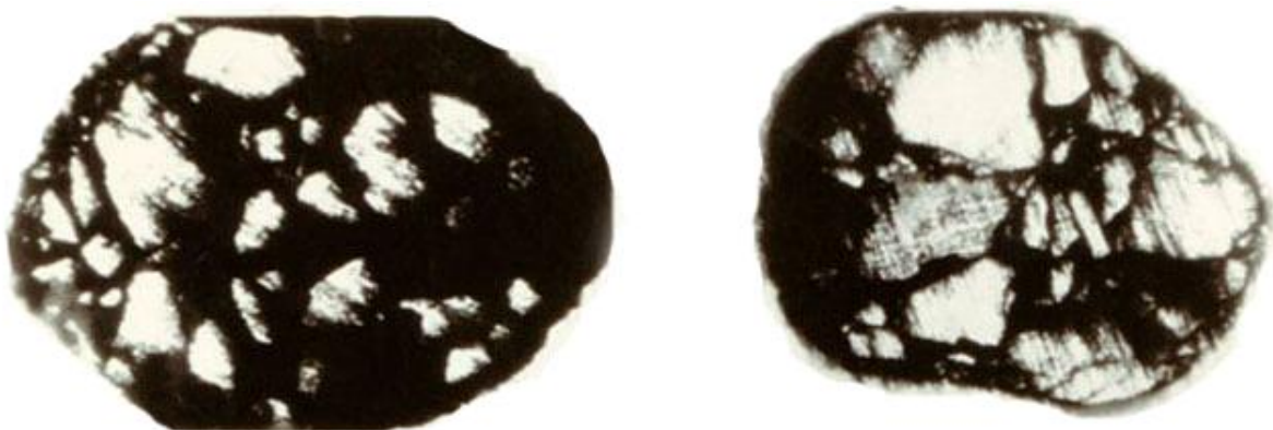
Fig.2. Anshlifs of granules: I type (a, b) - x600; III type(c,d,) - x400.
