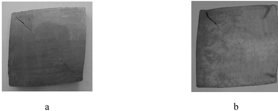
Figure 4 – Typical arrangement of longitudinal cracks on billets transversal templates (125 mm squares): a – 18 mm rhomboidity; b – 16 mm.
